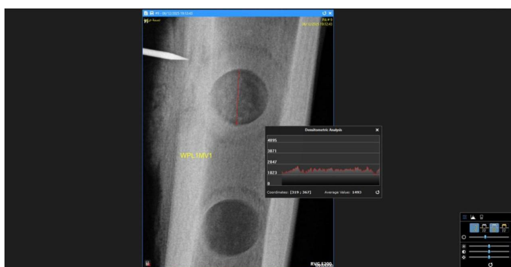
Fig. 4. Radiographic densitometric screenshot labelled WPL1MV1, showing a selected defect-related field with an average value of approximately 1493.
