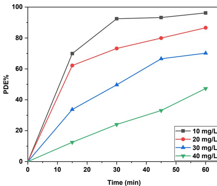
Fig. 9. removal percent BB dye at different initial concentration.
