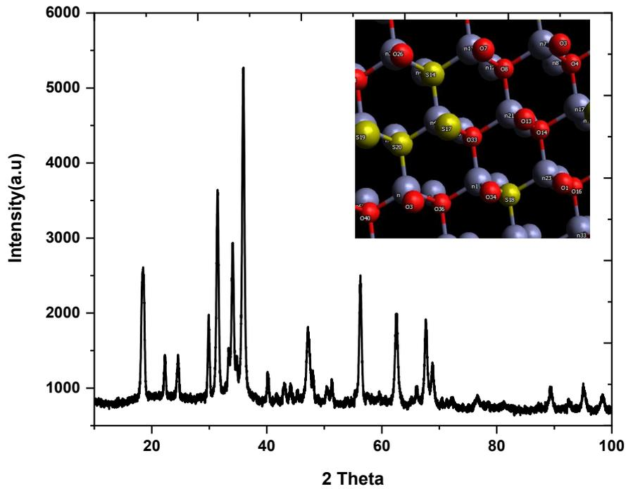
Fig. 5. XRD structure of ZnS/ZnO nanocomposite.
