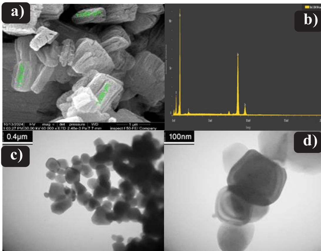
Fig. 4. FESEM images of a) ZnS/ZnO ;b) EDX of ZnS/ZnO; TEM c), d) of ZnS/ZnO NPs.
