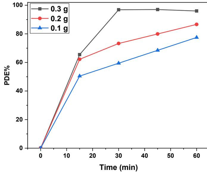
Fig. 7. Removal percentage of BB dye by ZnS/ZnO nanoparticles.
