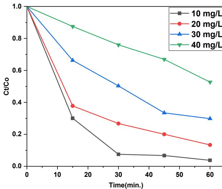
Fig. 8. Photocatalytic degradation at different concentration of BB dye onto ZnS/ZnO nanoparticles.
