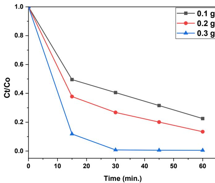
Fig. 6. Effect of the weight of ZnS/ZnO nanoparticles on photocatalytic degradation BB dye.
