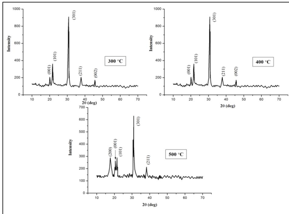
Fig. 2. XRD spectra of V<sub>2</sub>O<sub>5</sub> thinfilm at different substrate temperature.
