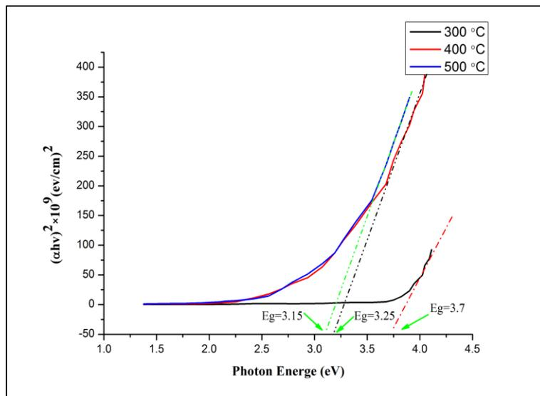
Fig. 5. The optical band gap of V<sub>2</sub>O<sub>5</sub> thin films deposited by different substrate temperatures.
