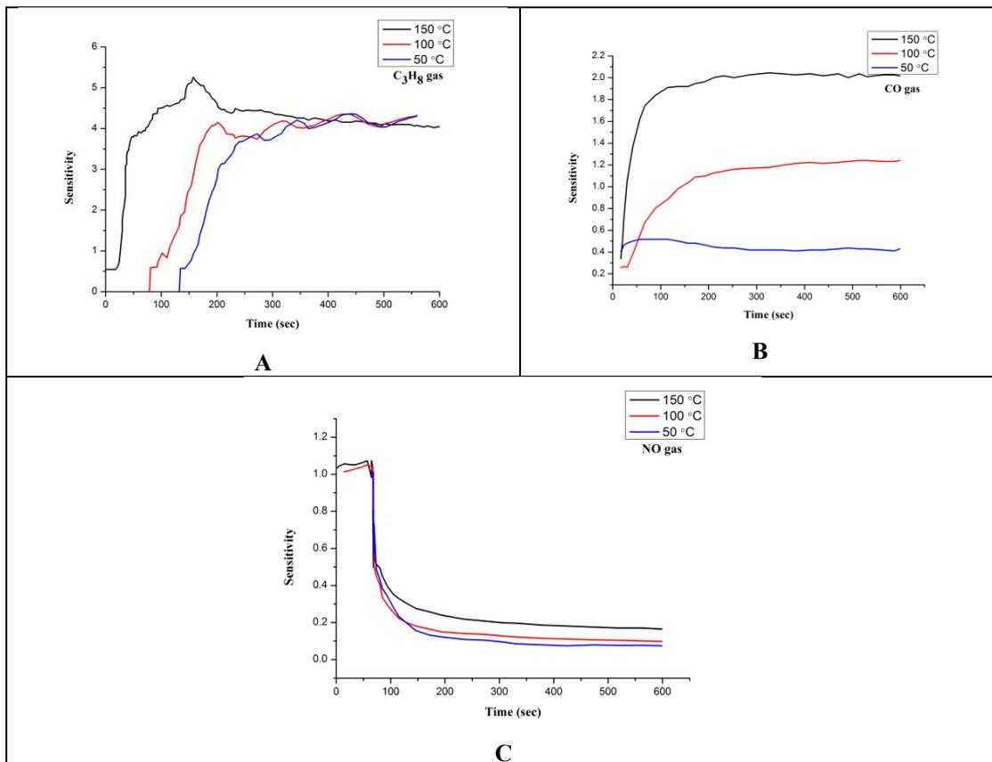
Fig. 6. Sensitivity properties of V<sub>2</sub>O<sub>5</sub> thin film sensors prepped at substrate temperature 400 °C for (a) C<sub>3</sub>H<sub>8</sub>, (b) CO and (c) NO gases.
