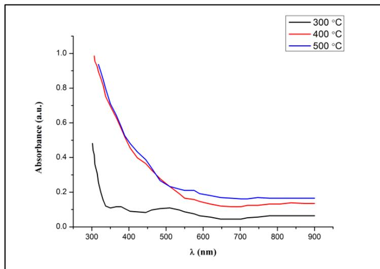
Fig. 4. Optical Absorbance versus wavelength for V<sub>2</sub>O<sub>5</sub> films with different substrate temperatures.
