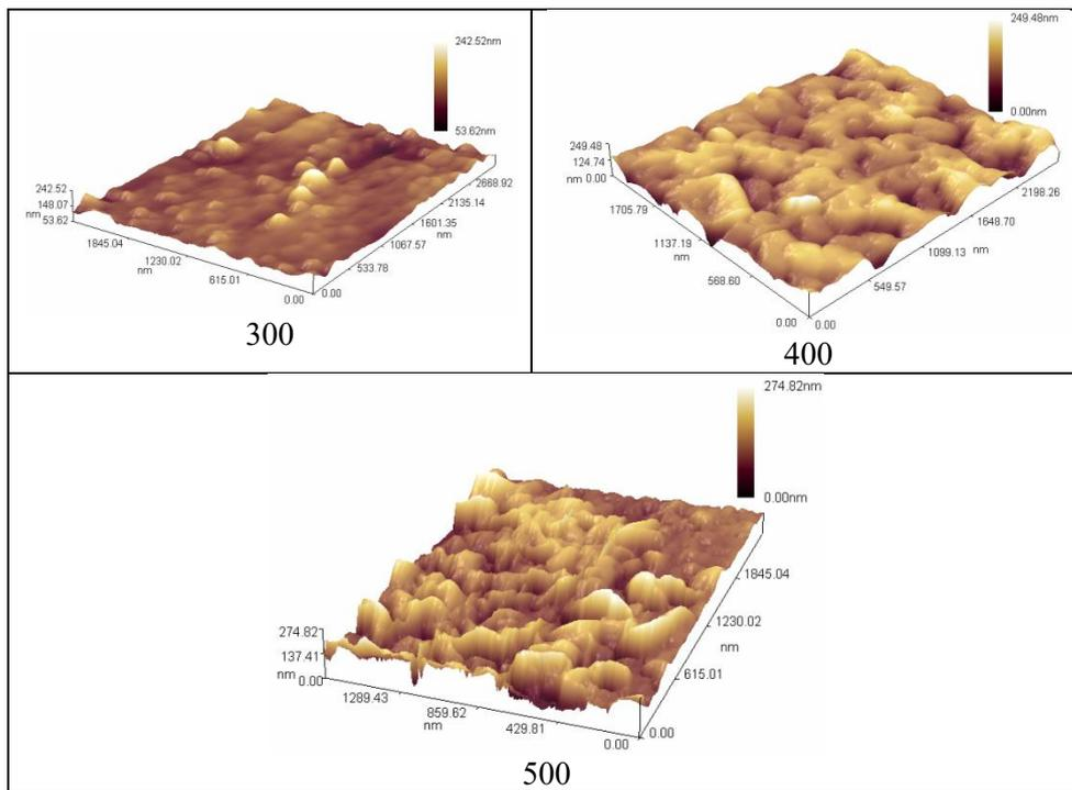
Fig. 3. AFM topographies of V<sub>2</sub>O<sub>5</sub> thinfilm at different substrate temperature.
