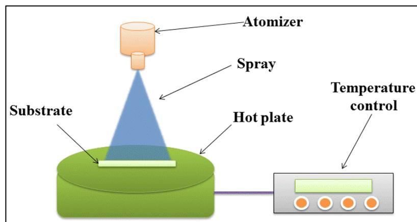
Fig. 1. Spray pyrolysis system diagram for preparation V<sub>2</sub>O<sub>5</sub> thin film.
