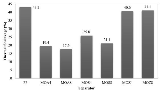
Fig. 4. Thermal shrinkages of the neat and the coated separators at 160 °C for 30 min.
