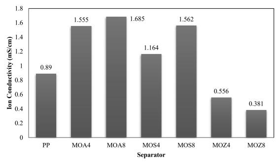
Fig. 8. Ion conductivities of the neat PP and the inorganic coated separators.
