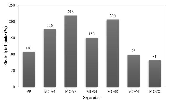
Fig. 7. Electrolyte uptakes of the neat PP and the coated separators.
