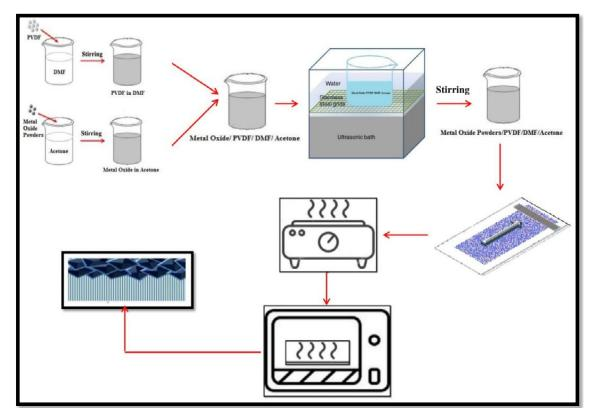
Fig. 1. Schematic representation of the separator's coating procedure.
