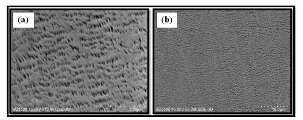
Fig. 2. SEM images of the neat PP separators with different magnification of: (a) 15.0 k, and (b) 3.00 k.
