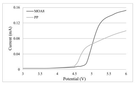
Fig. 9. Electrochemical stabilities of the PP and the MOA8 coated separators.
