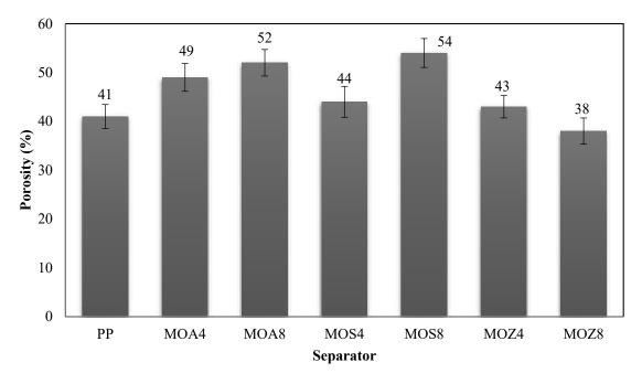
Fig. 5. The neat PP and the coated PP separators measured porosities.
