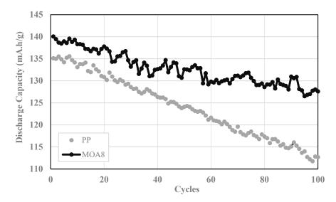
Fig. 10. Cycling performances of the LiFePO4 half cells equipped with the neat PP and the MOA8 coated separators.
