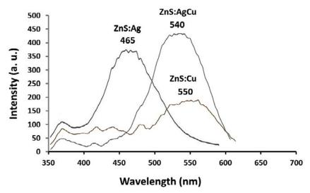
Fig. 6. The PL spectra of ZnS with Ag, Cu and AgCu impurities.
