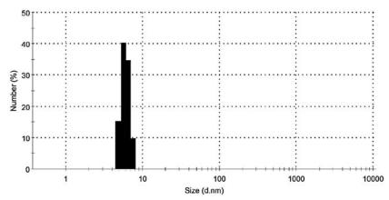
Fig. 5. Size distribution of prepared ZnS:Ag NPs obtained by DLS technique.
