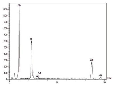
Fig. 2. The EDX spectrum of Ag-doped ZnS.
