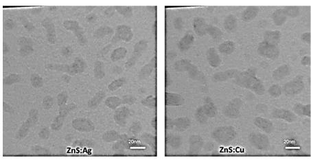
Fig. 4. The TEM image of produced ZnS:Ag and ZnS:Cu by hydrothermal method.
