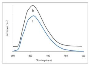
**Fig. 6.** Photoluminescence spectra of the synthesized  $\text{Li}_2\text{Si}_2\text{O}_5$  nanomaterials ( $\lambda_{ex} = 281$  nm), where a is  $S_1$  and b is  $S_2$ .
