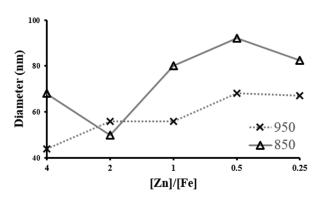
**Fig. 5**. Diagram of Average diameters of resulted carbon nanotubes using catalysts with the [Zn]/[Fe] proportion of 4, 2, 1, 0.5 and 0.25 at reaction temperatures of 850 and 950  $^{\circ}$ C.
