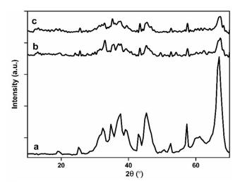
Fig. 2. XRD patterns of (a) alumina, (b) Zn<sub>4</sub>Fe, (c) Zn<sub>2</sub>Fe.
