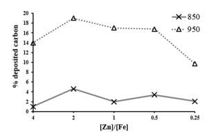
**Fig. 8.** Diagram of the weight loss percent of resulted carbon nanotubes using catalysts with the [Zn]/[Fe] proportion of 4, 2, 1, 0.5 and 0.25 at reaction temperatures of 850 and 950 °C.
