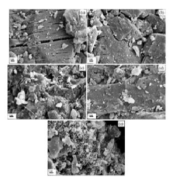
$\begin{aligned} \textbf{Fig. 3}. & \text{ SEM images of (a) } Zn_4NT_{850}\text{, (b) } Zn_4NT_{850}\text{, (c)} \\ & Zn_1NT_{850}\text{, d)}Zn_{0.5}NT_{850}\text{(e) } Zn_{0.25}NT_{850}. \end{aligned}$
