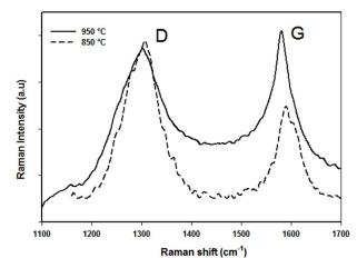
**Fig. 9.** Typical Raman spectra of  $Zn_2CNT_{950}$  and  $Zn_2CNT_{850}$ .
