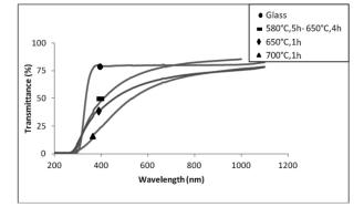
Fig. 8. The optical transmission spectra for glass, the samples prepared by two-step heat-treatment method (nucleated at 580 °C, 5 h and heated at 650 °C, 4 h), and the samples prepared by one-step heat-treatment method, 650 °C, 1 h and 700 °C, 1 h. The transparency of glass-ceramic is improved by two-step heat-treatment method.
