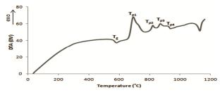
Fig. 1. DTA curve of the parent glass.
