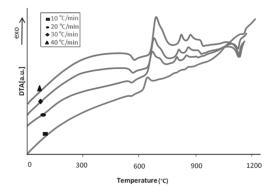
Fig. 9. DTA curves for glass sample recorded at different heating rates ranging from 10 to 40  $^{\circ}$ C /min.
