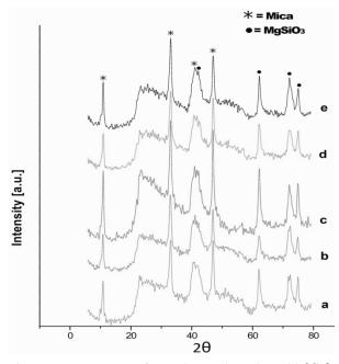
Fig. 5. XRD patterns of samples nucleated at 580  $^{\circ}$ C for (a) 1 h, (b) 3 h,( c) 5 h, (d) 7 h and (e) 9 h and heated at 650  $^{\circ}$ C for 4 h.
