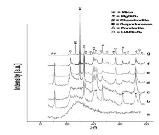
Fig. 2. XRD patterns of (a) glass and samples heated at: (b) 650 °C, 9(c) 700 °C, (d) 750 °C, (e) 800 °C, (f) 850 °C and (g) 900 °C for 1 h.
