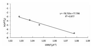
Fig. 11. Determination of crystallization activation energy.
