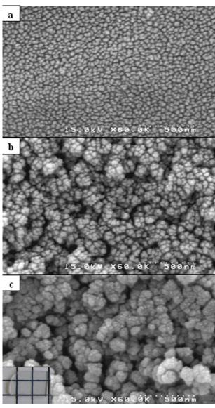
Fig. 6. SEM photographs of the samples a) glass, b) nucleated at 580  $^{\circ}$ C for 5 h and c) nucleated at 580  $^{\circ}$ C, 5 h and crystallized at 650  $^{\circ}$ C, 4 h, the glass-ceramics produced under optimum conditions has very good transparency.
