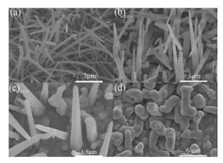
Fig. 5. SEM images of GeNWs with different ratio of Ar and  $H_2$  as carrier gas.
