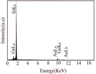
Fig. 4. EDS spectrum of the GeNWs with 80 sccm as carrier gas flow and catalyst of Au colloid solution.
