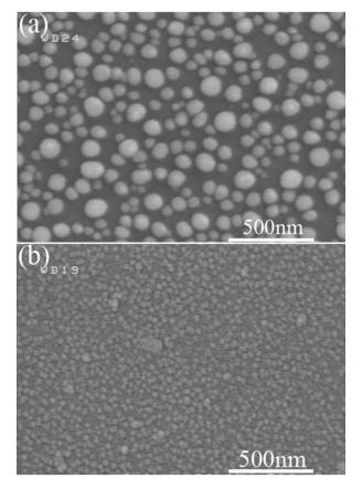
**Fig. 3.** SEM images of Au nanoparticles from (a) Au thin layer after annealing process at 500 C and (b) Au colloidal solution.
