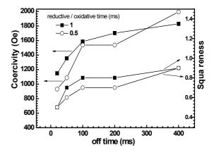
**Fig. 3.**Coercivity and squarenessas afunction of the off-time with reductive/oxidative times of 0.5 and 1 ms.
