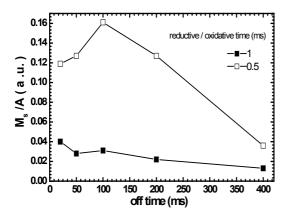
**Fig. 4.**Saturation magnetization per unit area as a function of the off-time using reductive/oxidative times of 0.5 and 1 ms.
