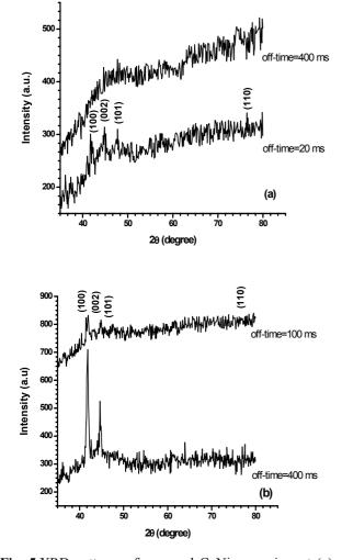
**Fig. 5.**XRD patterns of prepared CoNi nanowires at (a) reductive/oxidative time of 1 ms and off-time of 20, 400ms, (b) at reductive/oxidative time of 5ms and off-time of 100, 400ms.
