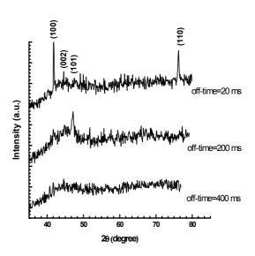
**Fig. 6.**XRD patterns of CoNi nanowire with reductive/oxidative time of 1.75ms.
