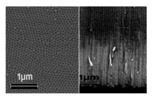
**Fig. 1.**(a) Top view SEM micrograph of porous Alumina template and (b) cross-section view SEM micrograph of CoNi-filled alumina template.
