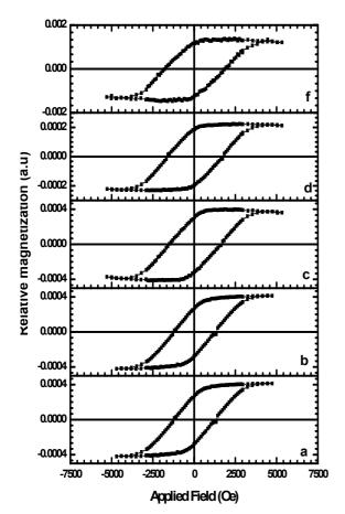
**Fig. 7.**The hysteresis loops of CoNi nanowire arrays with applied field parallel to the nanowire with the reductive oxidative time of 1ms and off-times of (a) 20ms, (b) 50ms, (c)100ms, (d) 200ms and (f) 400ms.
