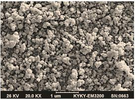
Fig. 4. SEM images of Fe<sub>3</sub>O<sub>4</sub>@SiO<sub>2</sub>@Mo-Schiff base.
