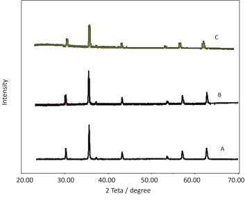
Fig. 3. XRD patterns of (A)  $Fe_3O_4$ , (B)  $Fe_3O_4$ @SiO<sub>2</sub> and (C)  $Fe_3O_4$ @SiO<sub>2</sub>@Mo-Schiff base.
