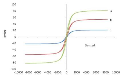
Fig. 6. VSM curves of (a) Fe<sub>3</sub>O<sub>4</sub>, (b) Fe<sub>3</sub>O<sub>4</sub>@SiO2 and (c) Fe<sub>3</sub>O<sub>4</sub>@SiO<sub>2</sub>@Mo-Schiff base.
