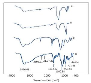
Fig. 2. FT-IR spectra of (A) Fe<sub>3</sub>O<sub>4</sub>@SiO<sub>2</sub> (B) Fe<sub>3</sub>O<sub>4</sub>@SiO<sub>2</sub>@APTES and (C) Fe<sub>3</sub>O<sub>4</sub>@ SiO<sub>2</sub>@Mo-Schiff base, (D) used Fe<sub>3</sub>O<sub>4</sub>@SiO<sub>2</sub>@Mo-Schiff base.
