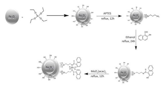
Fig. 1. Preparation of Fe<sub>3</sub>O<sub>4</sub>@SiO<sub>2</sub>@Mo-Schiff base
