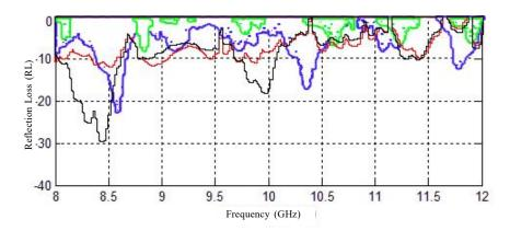
Fig. 6. The variations of RL versus frequency in the range of 8-12 GHz for A1 (green), A2
