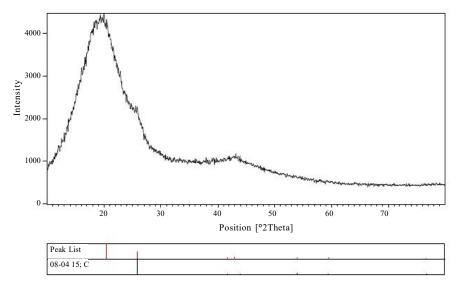
Fig. 5. XRD patterns of the CB/epoxy composites.
