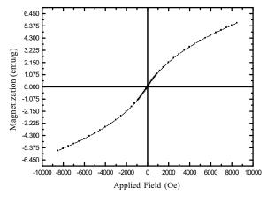
Fig. 8. AGFM of CoFe<sub>2</sub>O<sub>4</sub> nanoparticles.
