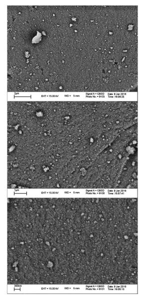
Fig. 3. SEM images of CoFe<sub>2</sub>O<sub>4</sub> nanoparticles at 400 ml of water (diluted sample)
