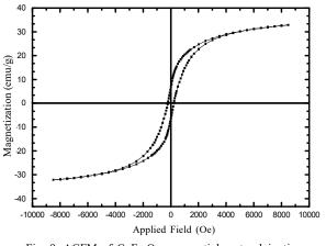
Fig. 9. AGFM of  $CoFe_2O_4$  nanoparticles at calcination temperature of 500 °C.
