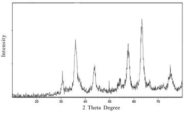
Fig. 1. XRD pattern of CoFe<sub>2</sub>O<sub>4</sub> nanoparticles
