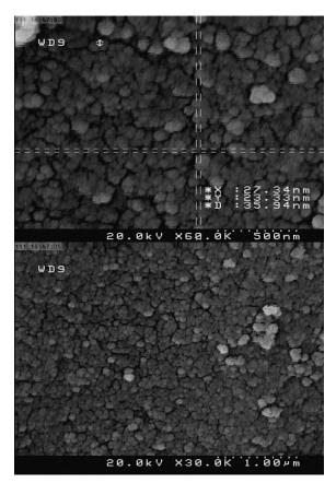
Fig. 2. SEM images of surfactant-free CoFe<sub>2</sub>O<sub>4</sub> nanoparticles
