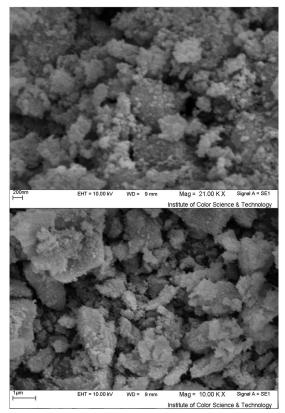
Fig. 6. SEM image of  ${\rm CoFe_2O_4}$  nanoparticles synthesized by cobalt acetate
