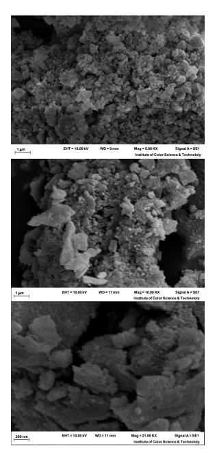
Fig. 5. SEM image of  $\mathrm{CoFe_2O_4}$  nanoparticles synthesized by starch
