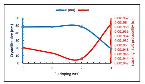
Fig. 2. Crystalline size and stacking fault probability of NiO: Cu films with Cu-doping ratios.
