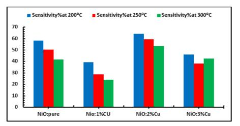
Fig. 12. Histogram of the sensitivity% values of NiO: Cu films for NO<sub>2</sub> gas.
