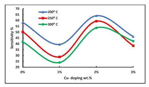
Fig. 8. The sensitivity of NiO:Cu films with Cu concentration at different operating temperatures for NO<sub>2</sub> gas.
