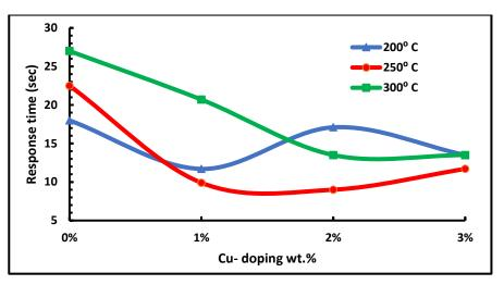
Fig. 9. Response time of NiO: Cu films for H<sub>2</sub>S gas.
