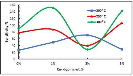
Fig. 7. The sensitivity of NiO:Cu films with Cu concentration at different operating temperatures for  $H_2S$  gas.
