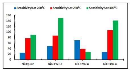
Fig. 11. Histogram of the sensitivity% values of NiO: Cu films for H<sub>2</sub>S gas.
