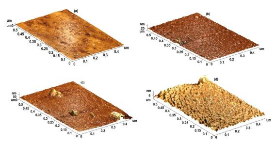
Fig. 3. AFM images NiO: Cu films, (a) 0%Cu-doped, (b) NiO:1%Cu-doped, (c) NiO:2%Cu-doped, (d) NiO:3%Cu-doped.
