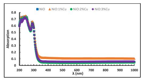
Fig. 5. UV- Visible absorption diagrams of the NiO: Cu films at different Cu-doping.
