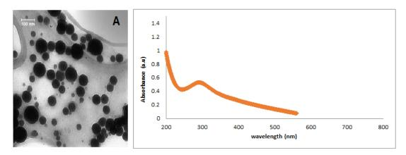
Fig. 3. A) TEM of spherical shaped colloidal synthesis of selenium nanoparticles in aqueous rosemary extract (CSSNANO). B) UV–visible absorption spectrum of the CSSNANO suspension
