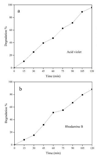
Fig. 7: Photocatalytic activity of  $CuO/CeO_2$  nanocomposites against a) Acid violet 7 b) Rhodamine B.
