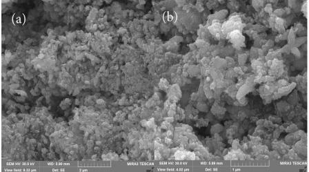
Fig. 6. SEM images of Cu doped ZnS nanoparticles
