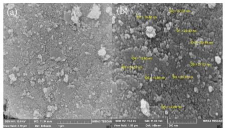
Fig. 7. SEM images of  $CoFe_2O_4$ -ZnS-Ag-doped nanocomposite
