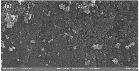
Fig. 2. SEM images of cobalt ferrite nanoparticles
