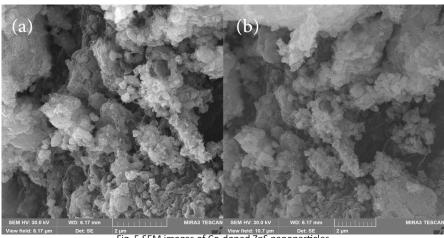
Fig. 5.SEM images of Co-doped ZnS nanoparticles
