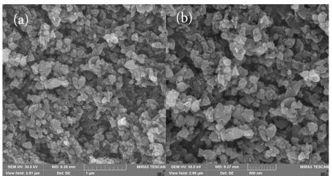
Fig. 3. SEM images of Ag-doped ZnS nanoparticles
