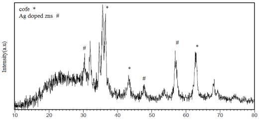
Fig. 1. XRD pattern of CoFe<sub>2</sub>O<sub>4</sub>-ZnS-Ag-doped nanocomposite
