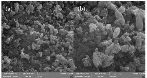
Fig. 4. SEM images of Ni-doped ZnS nanoparticles
