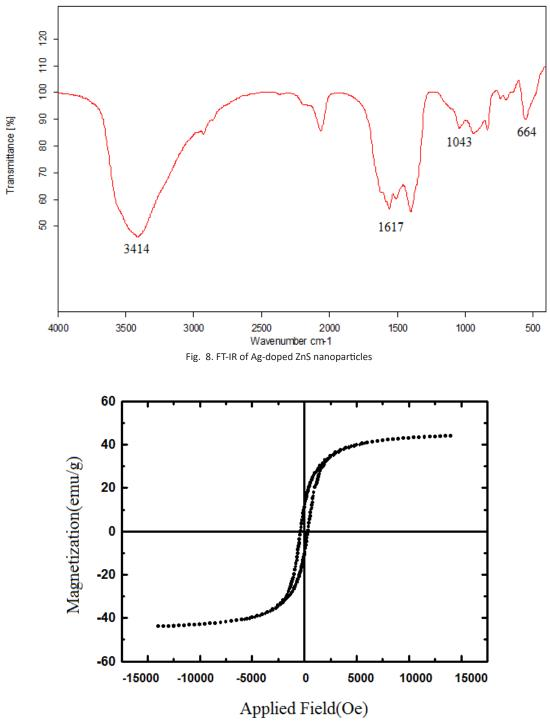
Fig. 9. AGFM curve of CoFe<sub>2</sub>O<sub>4</sub>-ZnS-Ag-doped nanocomposite
