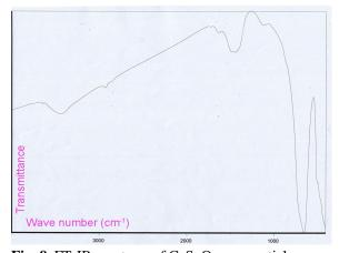
Fig. 9. FT-IR spectrum of CaSnO<sub>3</sub> nanoparticles
