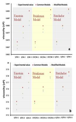
Fig. 3. Deviation of models and modified models with experimental viscosity of a) water base NF b) EG base NFs
