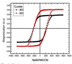
**Fig. 9.** The hysteresis loops of as-prepared samples with 360 CoFe pulse and 200, 400 Cu pulse.
