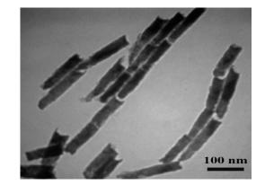
**Fig. 2.** TEM image of CoFe/Cu multilayer nanowires with 300 Cu pulses and 410 CoFe pulses.
