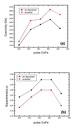
**Fig. 5.** (a) coercivity ( $H_c$ ) and (b) The squareness ( $S_q$ ) of prepared and annealed samples as a function of CoFe pulses.
