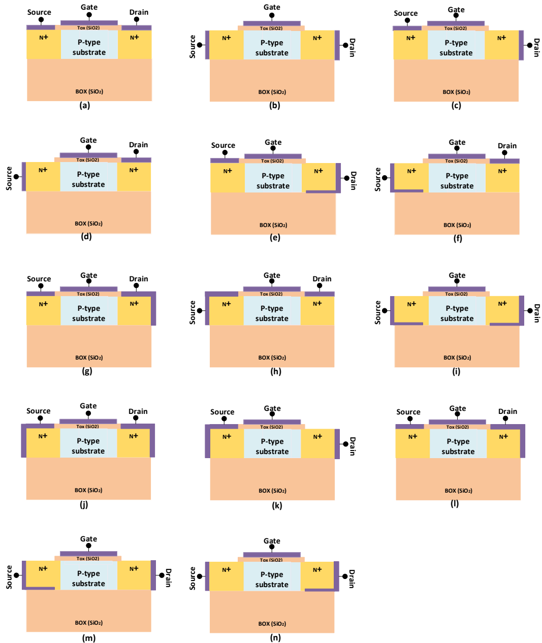
Fig. 1. Different source and drain electrodes geometry considered in this research.
