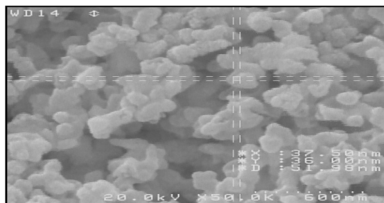
Fig. 6. SEM photographs of \text{Co}_3\text{O}_4 nanoparticles produced by calcination of precursor 1 at 550°C.
