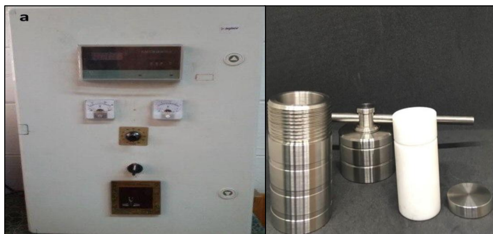
Fig. 1. Hydrothermal system. a) Temperature control unit b) The Reactor which consists of Teflon lined autoclave.
