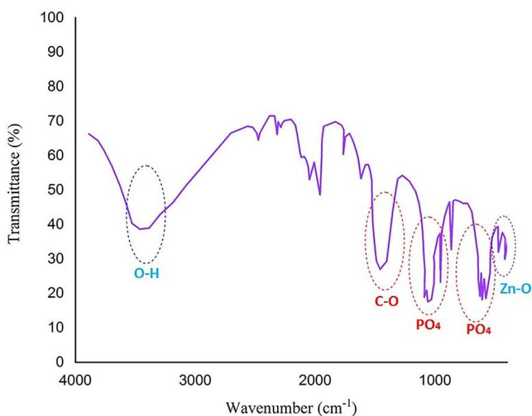
Fig. 2. FT-IR analysis of ZnO/hydroxyapatite composite.
