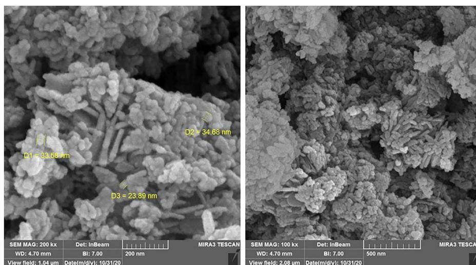
Fig. 3. The FE-SEM images of the ZnO/hydroxyapatite composite.
