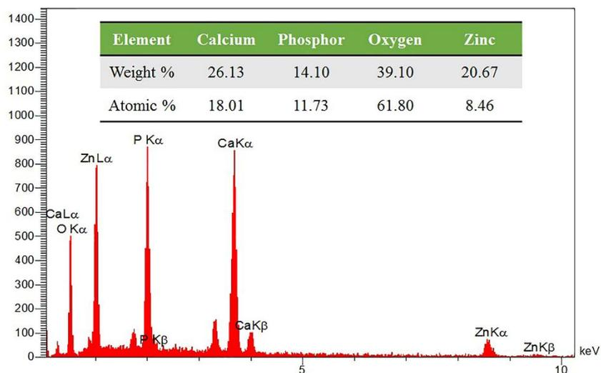
Fig. 4. The EDX pattern of ZnO/hydroxyapatite composite.
