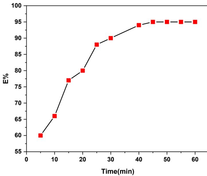
Fig. 5. Effect of Contact Time on the removal GRL dye by hydrogel nanocomposite.
