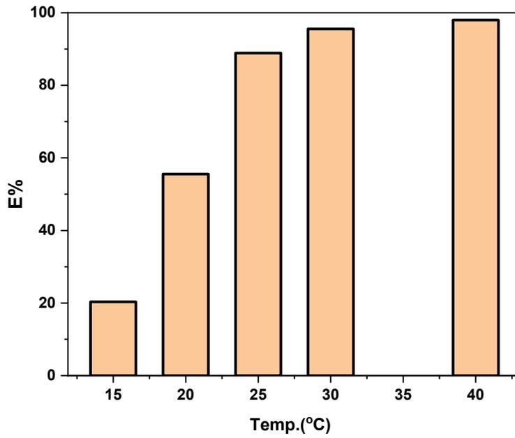
Fig. 6. Effect of Temperature on the removal GRL dye by hydrogel nanocomposite.
