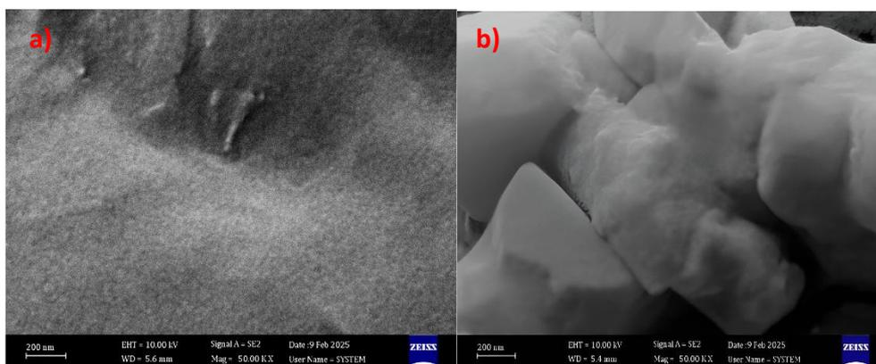
Fig. 1. FESEM image of a) hydrogel before adsorption, b) hydrogel after adsorption.
