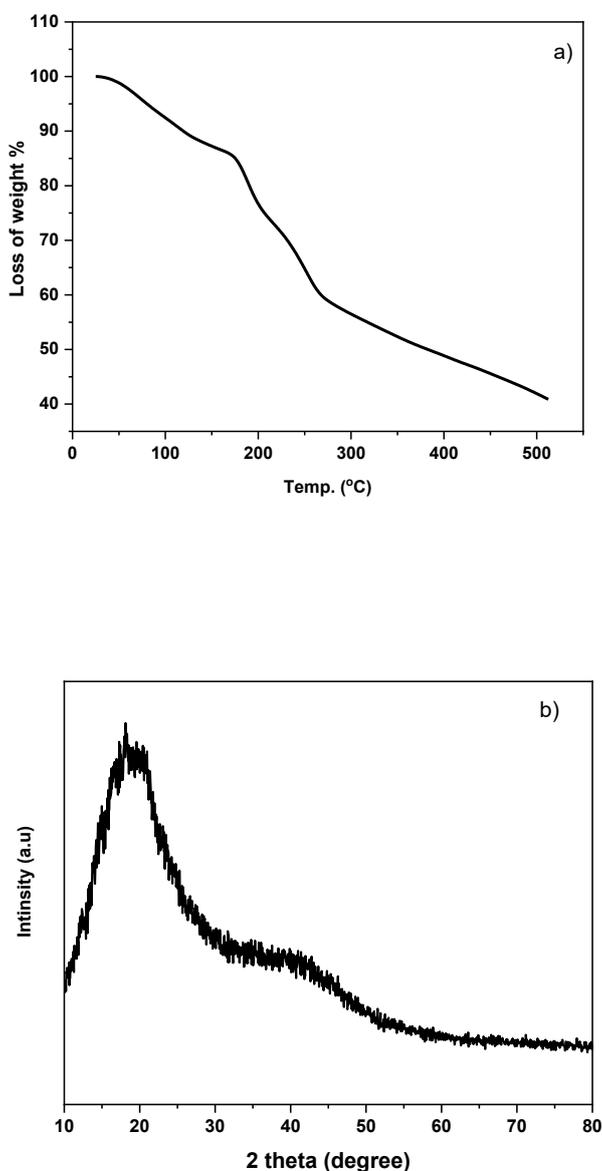
Fig. 3. a) TGA of hydrogel nanocomposite, b) XRD of hydrogel nanocomposite.
