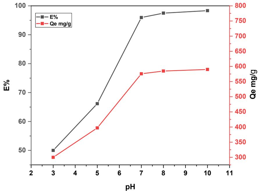
Fig. 7. Effect of pH solution on the removal GRL dye by hydrogel nanocomposite.
