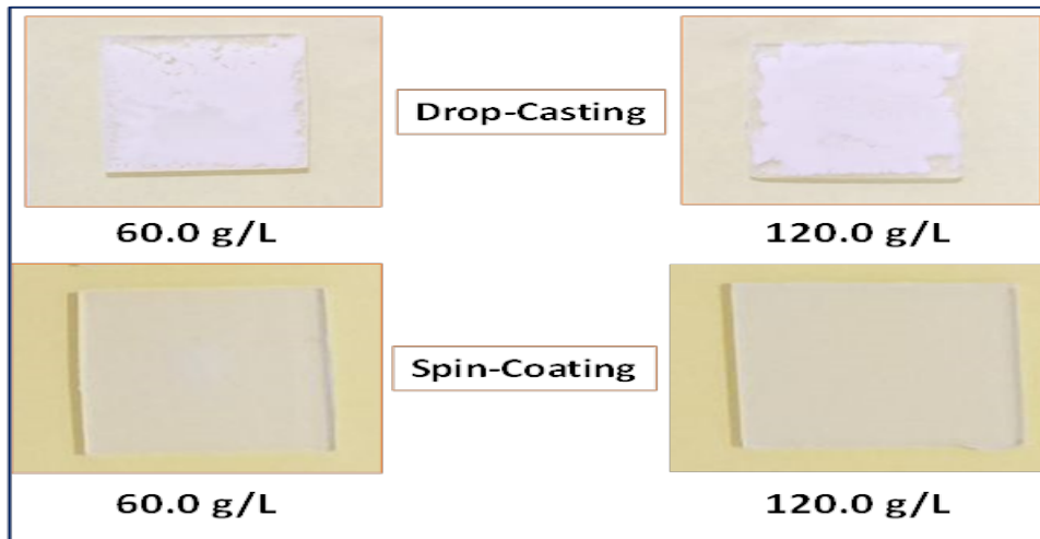
Fig. 4. Images of glass surface coated with TiO 2 at two solution concentrations
