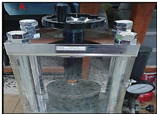
Fig. 1. (A) The pressure system used to compress research samples. (B) A picture of the sample prepared for the mixtures with equal weight ratios in this work after the pressing process
