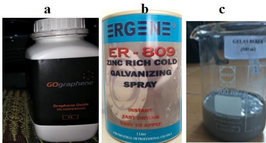
Fig.1 a) Graphene oxide, b) Galvanized and c) Mixture of GO and Galvanized sample.
