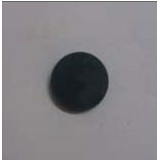
Fig. 13. Sintered NiO-based nanocrystalline ceramic composite oxide pellet
