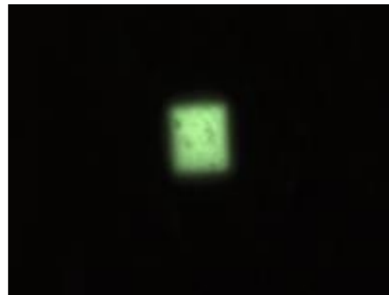
Fig. 8. Ion beam induced luminescence (IBIL) of Gd_2O_3:S:Tb^{3+} layer
