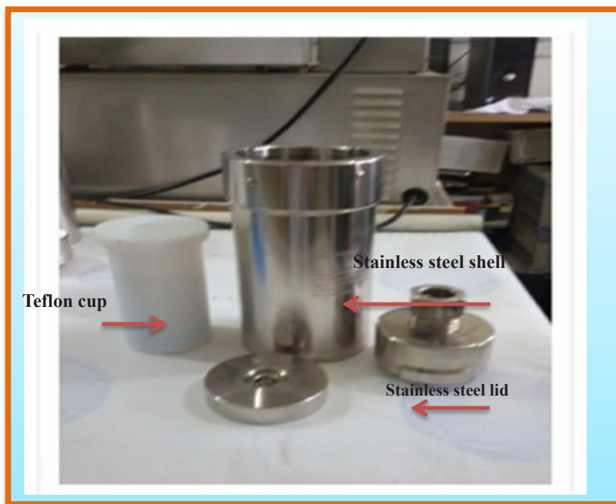
Fig. 1. Real image of autoclave with main compound, college of science for Women- University of Babylon.
