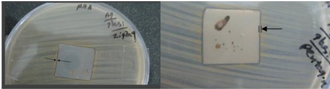
Fig. 4. typical zone of inhibition (ZOI) for L-shaped (left) and HP(right) sculptured thin films on Petri dish for E. coli ATCC 8739 bacteria, after 24 hours incubation.
