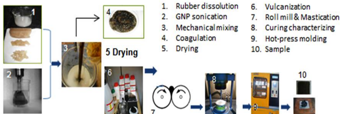
Fig. 1. Steps of preparation vulcanized (GNP/NBR) rubber nanocomposite
