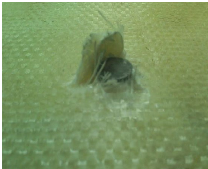
Fig. 9. Fragmentation of composite parts in the test
