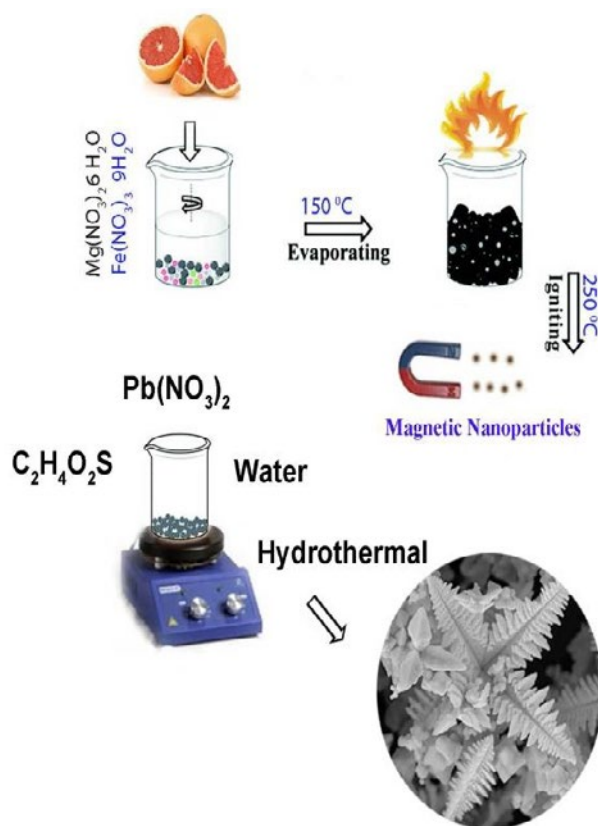
Fig. 1. Preparation mechanism of the magnetic product and star like PbS.
