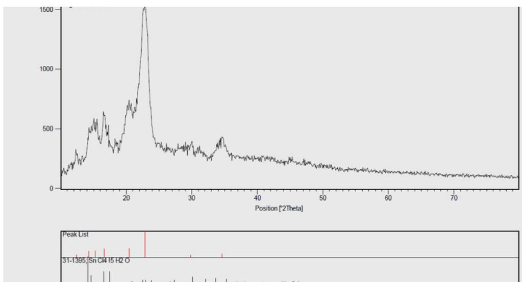
Fig. 6. XRD pattern of  $\text{SnCl}_4/\text{nano-sawdust}$
