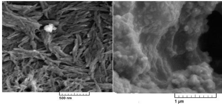
Fig. 4. The FESEM image of (a) nano-sawdust and (b)  $\text{SnCl}_4/\text{nano-sawdust}$ .
