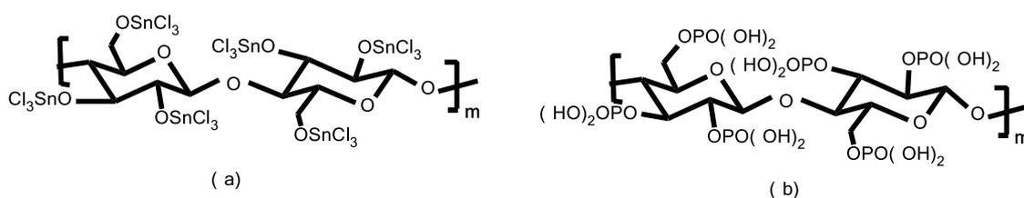
Fig. 3. Proposed structure for (a) SnCl<sub>4</sub>/nano-sawdust and (b) cellulose triphosphate.
