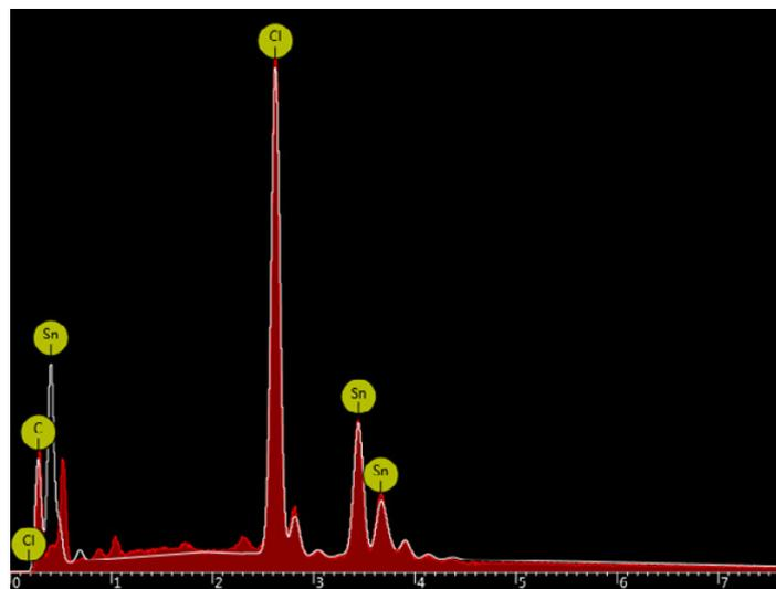
Fig. 5. EDS analysis diagram of  $\text{SnCl}_4/\text{nano-sawdust}$ .
