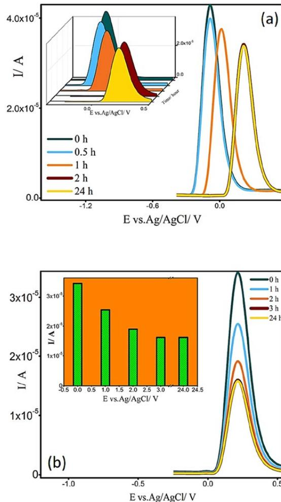
Fig. 7. Optimizing the immobilization time of APTA/Bio AuNP/ Pol/ Cu<sub>2</sub>O\_CD / SPE (a) and the hybridization time of Anti/ APTA/Bio AuNP/ Pol/ Cu<sub>2</sub>O\_CD / SPE (b) in 2 mM of catechol in PBS.
