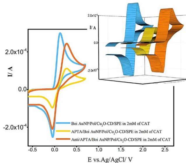
Fig. 4. Detecting of the immobilization and hybridization process at Bio AuNP/ Pol/ Cu<sub>2</sub>O\_CD / SPE and APTA/Bio AuNP/Pol/Cu<sub>2</sub>O\_CD/SPE, respectively, in 2 mM of catechol in PBS.
