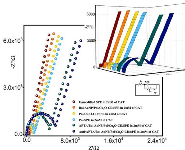
Fig. 5. Nyquist plots of SPE, Pol/ SPE, Pol /Cu<sub>2</sub>O\_CD / SPE, Bio AuNP/ Pol/ Cu<sub>2</sub>O\_CD / SPE APTA/Bio AuNP/ Pol/ Cu<sub>2</sub>O\_CD / SPE, Anti/APTA/Bio AuNP/ Pol/ Cu<sub>2</sub>O\_CD / SPE in 1 mM of [Fe(CN)<sub>6</sub>]<sup>3-/4-</sup> in PBS. Inset: Equivalent circuit for fitting the plots.
