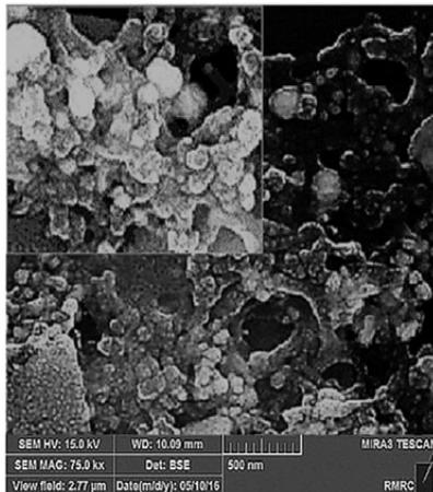
Fig. 2. A SEM micrograph of the biosynthesized gold nanoparticles.
