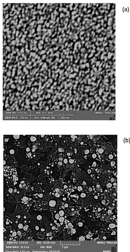
Fig. 1. A SEM micrograph of the carbon dot (CD) (a) and Cu<sub>2</sub>O\_CD (b).
