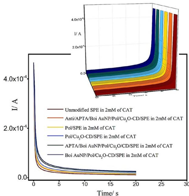
Fig. 6. Chronoamperometric results, obtained at SPE, Pol/ SPE, Pol/ $\text{Cu}_2\text{O}$ \_CD / SPE, Bio AuNP/ Pol/  $\text{Cu}_2\text{O}$ \_CD / SPE, APTA/Bio AuNP/ Pol/  $\text{Cu}_2\text{O}$ \_CD / SPE, Anti/ APTA/Bio AuNP/ Pol/  $\text{Cu}_2\text{O}$ \_CD / SPE in 2 mM of catechol in PBS.
