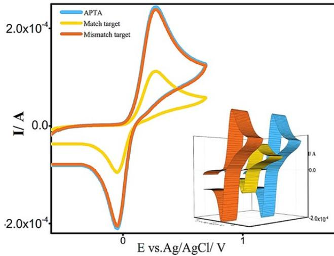
Fig. 8. Detecting of the selectivity of APTA/Bio AuNP/ Pol/ Cu<sub>2</sub>O\_CD / SPE in 2 mM of catechol in PBS.
