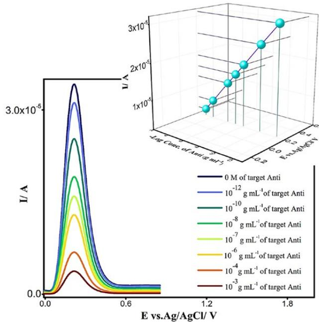
Fig. 9. DPVs of Anti/APTA/Bio AuNP/ Pol/ Cu<sub>2</sub>O\_CD / SPE in 2 mM of catechol in PBS, at different concentrations of target antigen (CEA).
