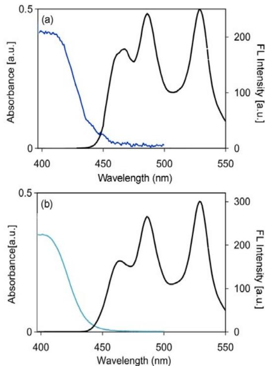
Fig. 6. UV-Vis and fluorescence spectra of (a) L- and (b) D-cyst-CdS-QDs. Excitation wavelength for all fluorescence spectra is 388 nm.
