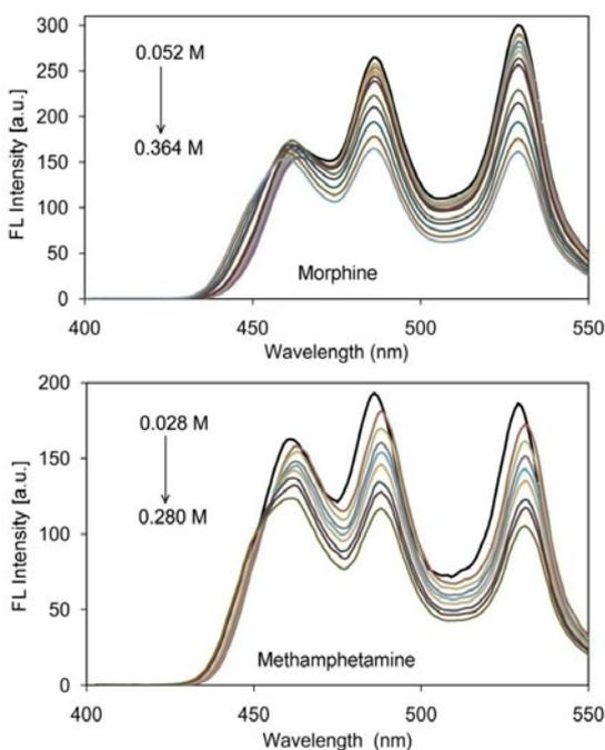
Fig. 7. The fluorescence spectra of L-cyst-CdS-QDs upon addition of the various concentrations of L-morphine and D-methamphetamine.
