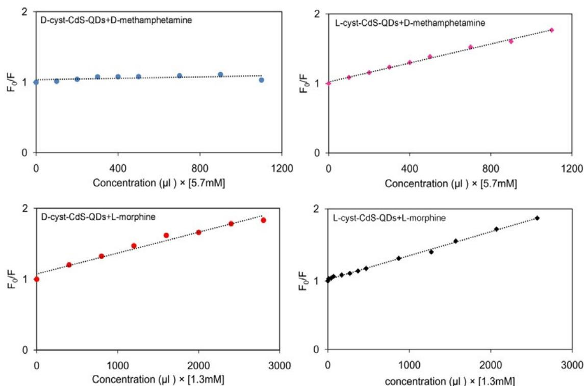
Fig. 9. Stern-Volmer plots of interaction between L- and D-cyst-CdS-QDs and L-morphine and D-methamphetamine.
