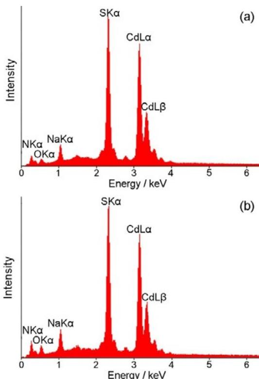
Fig. 4. EDX spectra of (a) L- and (b) D-cyst-CdS-QDs.
