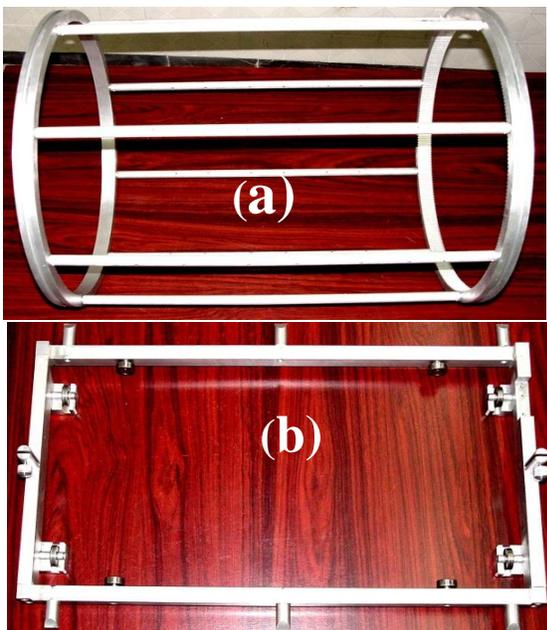
Fig. 3. (a) Substrate holder and (b) its stage.
