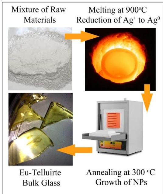
**Fig. 1.** Schematic steps of the glass preparation by the melt-quenching technique.
