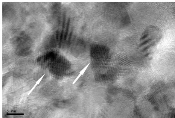
**Fig. 3.** TEM image of sample C. Few NPs are pointed by arrows. The scale bar is 5 nm.
