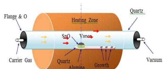
**Fig. 1.** Experimental set-up for synthesis of  $\text{SnO}_2$  nanowires.
