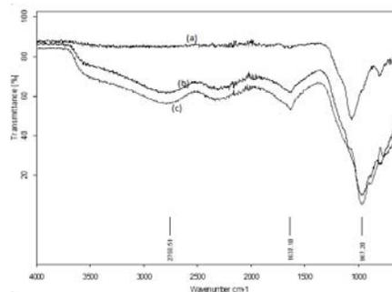
**Fig. 2.** ATR of a) silica chloride, b) nano-SPA and c)  $\text{H}_3\text{PO}_4 \cdot \text{SiO}_2$
