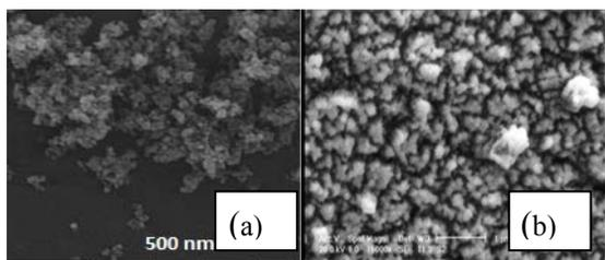
**Fig. 1.** The SEM photograph of a) nano silica-gel and b) nano-SPA.
