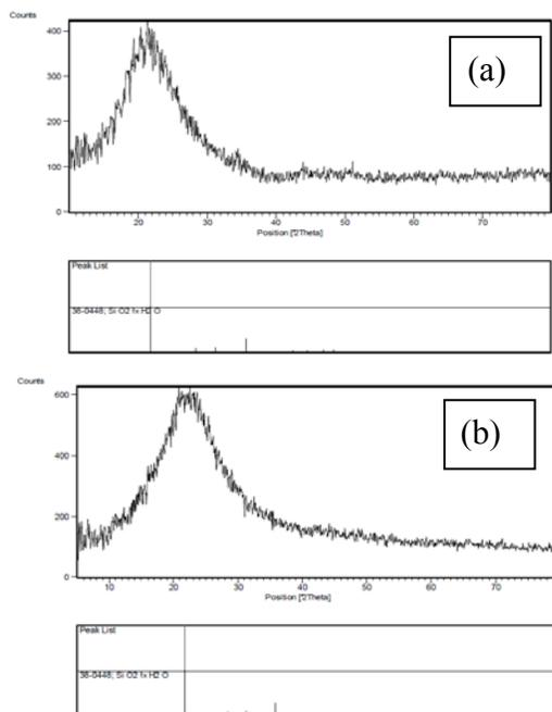
**Fig. 3.** : X-ray diffraction (XRD) pattern of a) nano SiO<sub>2</sub> and b) nano-SPA.
