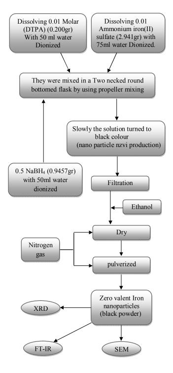
**Fig. 2.** Producing chart of zero valen Iron nano particles By Diethylene Triamine Penta Acetic acid (DTPA) Chelating Agent.
