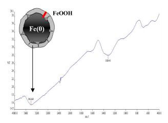
Fig. 6. FT-IR Spectrum of Synthesized NZVI.
