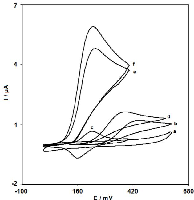
**Fig. 3.** CVs of (a) unmodified CPE in 0.1 M phosphate buffer solution (pH 7.0) at scan rate of  $10 \text{ mV s}^{-1}$ ; (b) as (a) + 0.1 mM EP; (c) as (a) at the surface of DDP-CNPE; (d) as (b) at the surface of CNPE; (e) as (b) at the surface of DDP-CPE; (f) as (b) at the surface of DDP-CNPE.
