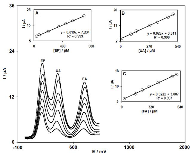
**Fig. 6.** DPVs of DDP-CNPE in 0.1 M phosphate buffer solution (pH 7.0) containing different concentrations of EP+UA+FA in  $\mu\text{M}$ , from inner to outer: 40.0+10.0+30.0, 75.0+100.0+150.0, 200.0+150.0+225.0, 350.0+275.0+300.0, 450.0+350.0+400.0, 550.0+450.0+550.0 and 700.0+500.0+600.0, respectively. Insets (A) (B) and (C) are plots of  $I_{pa}$  vs. EP, UA and FA concentrations, respectively.
