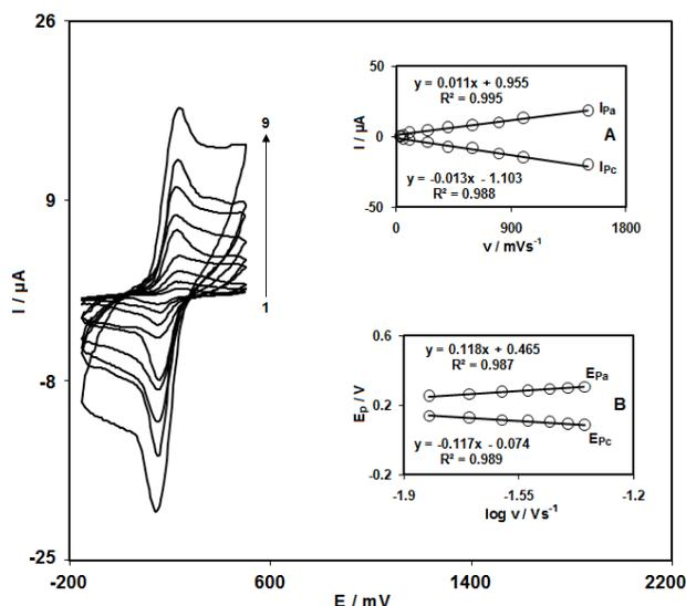
**Fig. 2.** CVs of DDP-CNPE in 0.1 M phosphate buffer (pH 7.0), at various scan rates, from inner to outer, 25, 50, 100, 250, 400, 600, 800, 1000 and 1500  $\text{mV s}^{-1}$ . Insets: variation of (A)  $I_p$  vs. scan rate; (B)  $E_p$  vs. the logarithm of high scan rates.
