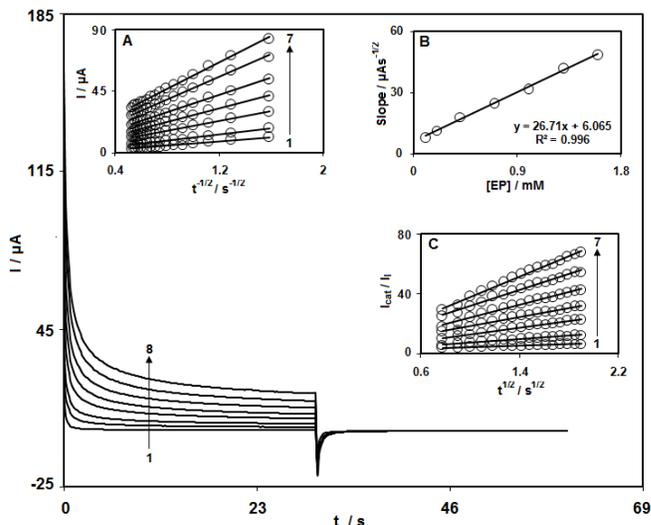
**Fig. 5.** Chronoamperograms obtained at DDP-CPE in 0.1 M phosphate buffer solution (pH 7.0) for different concentrations of EP. The numbers 1–8 correspond to 0.0, 0.1, 0.2, 0.4, 0.7, 1.0, 1.3 and 1.6 mM of EP. Insets: (A) Plots of  $I$  vs.  $t^{-1/2}$  obtained from chronoamperograms 2–8. (B) Plot of the slope of the straight lines against EP concentration. (C) Dependence of  $I_{\text{cat}}/I_1$  on  $t^{-1/2}$  derived from the data of chronoamperograms 1–8.
