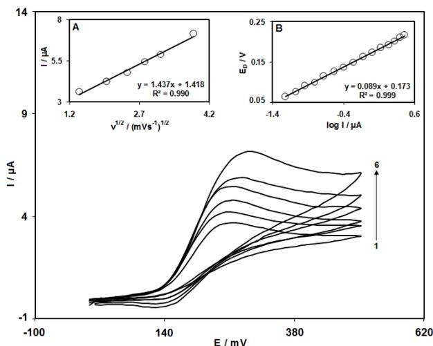
**Fig. 4.** CVs of DDP-CNPE in 0.1 M phosphate buffer solution (pH 7.0) containing 100.0  $\mu\text{M}$  EP at various scan rates; The numbers 1-6 correspond to scan rates of 2, 4, 6, 8, 10 and 15  $\text{mV s}^{-1}$ , respectively. Insets: variation of (A) anodic peak current vs.  $v^{1/2}$ ; (B) Tafel plot derived from the rising part of the voltammograms recorded at the scan rates of 10  $\text{mV s}^{-1}$ .
