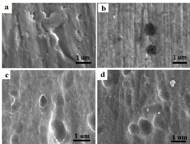
**Fig. 10.** SEM micrographs of abraded AA5052 (image a) pre-treated AA5052 after corrosion (image b), PANI coating after corrosion (image c) and PANI-Fe<sub>2</sub>O<sub>3</sub> nanocomposite coatings grown by an applied current density of 25 mA cm<sup>-2</sup> after corrosion (image d).
