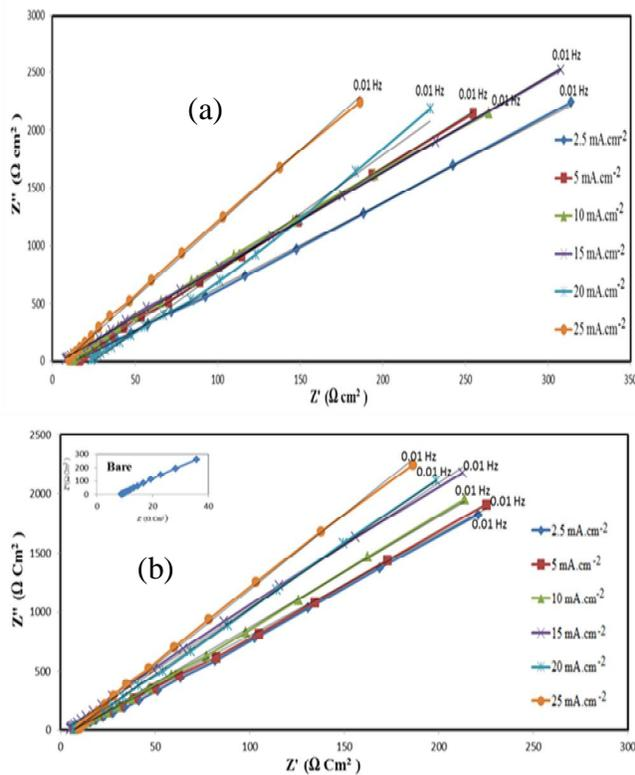
**Fig. 8.** Nyquist impedance plots for uncoated AA5052, (a) PANI and (b) PANI- Fe<sub>2</sub>O<sub>3</sub> coated AA5052 synthesized under galvanostatic conditions at various current densities (mA cm<sup>-2</sup>).
