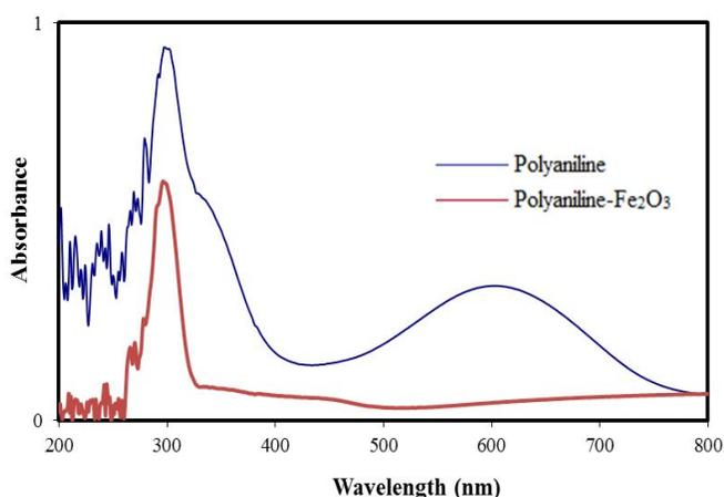
**Fig. 2.** UV-Vis spectrum recorded for the electrosynthesized pure PANI and PANI- $\text{Fe}_2\text{O}_3$  nanocomposite on the AA5052 electrode.
