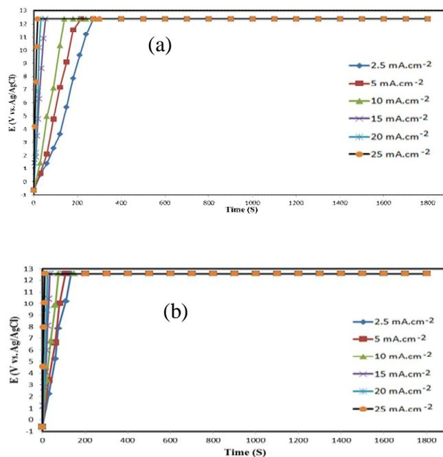
**Fig. 1.** E-t curve under galvanostatic polymerization conditions in 0.5 l (a) acetic acid solution containing (a) 0.1 M aniline and (b) 0.1 M aniline and 1 wt% dispersed Fe<sub>2</sub>O<sub>3</sub> nanoparticles for AA5052 electrode at various current densities (mA cm<sup>-2</sup>).
