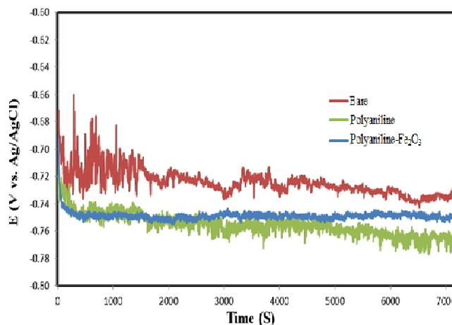
**Fig. 6.** OCP plots PANI and PANI-Fe $_2$ O $_3$  of coated AA5052 during 2 h immersion in 3.5% NaCl.
