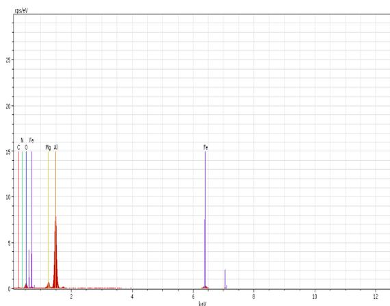
**Fig. 5.** EDX pattern of the electrosynthesized PANI-Fe $_2$ O $_3$  nanocomposite coated AA5052 for 25 mA cm $^{-2}$ .
