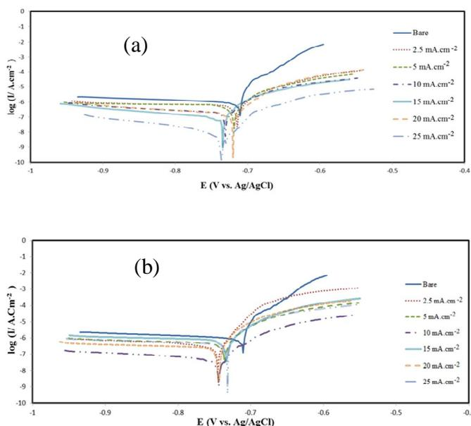
**Fig. 7.** Polarization behavior of electropolymerized (a) PANI, (b) PANI-Fe<sub>2</sub>O<sub>3</sub> nanocomposite-coated on AA5052 at various current densities (mA cm<sup>-2</sup>) in 3.5% NaCl.
