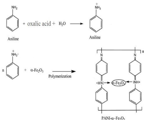
**Fig. 4.** The structure of PANI -Fe $_2$ O $_3$
