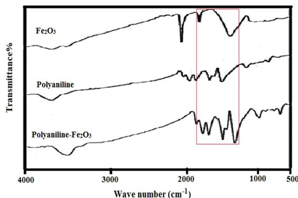
**Fig. 3.** FT-IR spectrum (a)  $\text{Fe}_2\text{O}_3$  nanoparticles (b) PANI and (c) the PANI- $\text{Fe}_2\text{O}_3$  nanocomposite.
