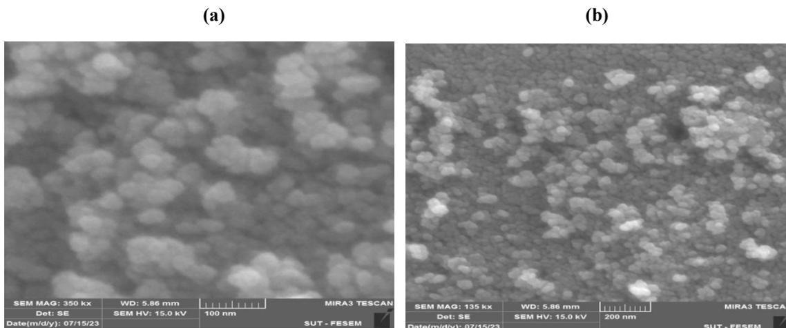
Fig. 4. FE-SEM images of  $\alpha$ -Fe<sub>2</sub>O<sub>3</sub> NPs.
