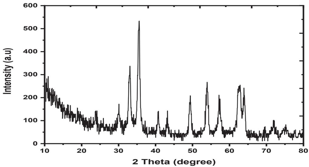
Fig. 1. XRD of α - Fe<sub>2</sub>O<sub>3</sub> NPs.
