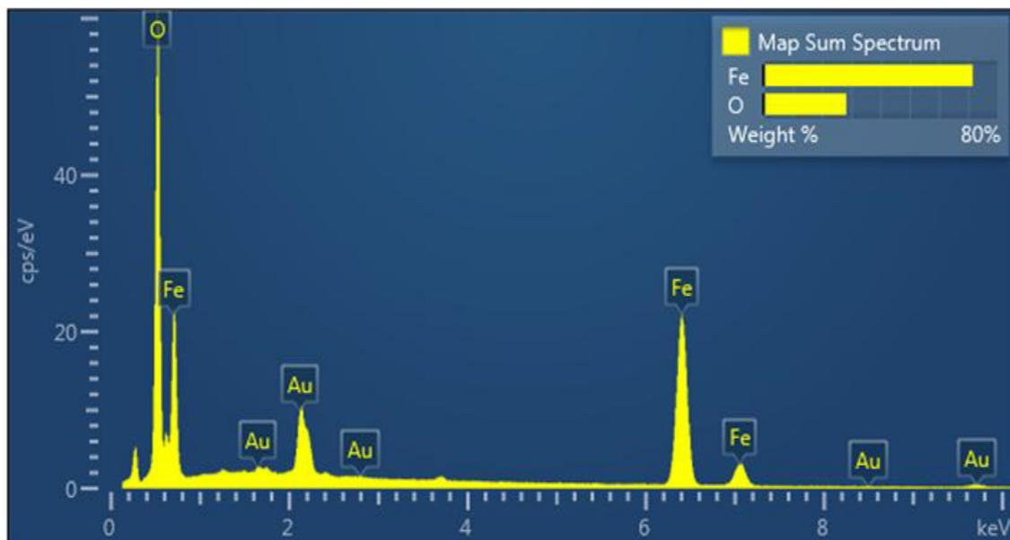
Fig. 2. EDX of α - Fe<sub>2</sub>O<sub>3</sub> NPs
