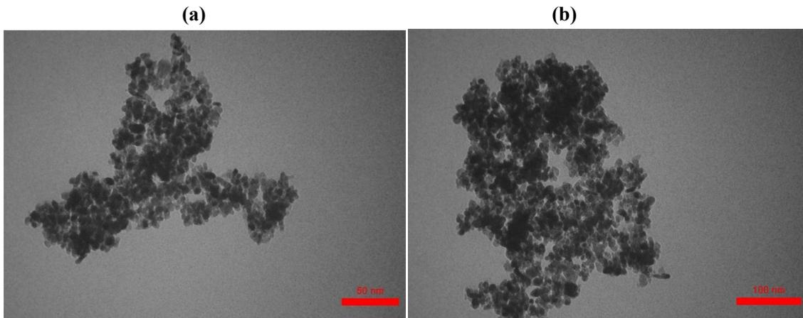
Fig. 3. TEM images of  $\alpha$ -Fe<sub>2</sub>O<sub>3</sub> NPs.
