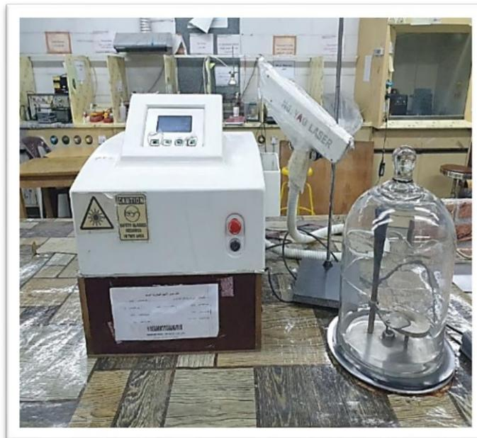
Fig. 1. Illustrate the parts of the PLD system
