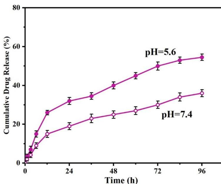
Fig. 5. In-vitro release pattern of quercetin from SCh-Qur@BSA-FA carrier at acidic and natural media.
