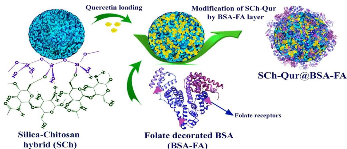
Fig. 1. overall steps of the preparation and structure of the SCh-Qur@BSA-FA nanocarrier.
