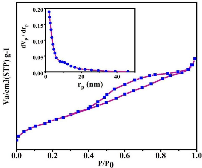
Fig. 3. Nitrogen adsorption-desorption isotherm of SCh-Qur@BSA-FA hybrid nanocarrier.
