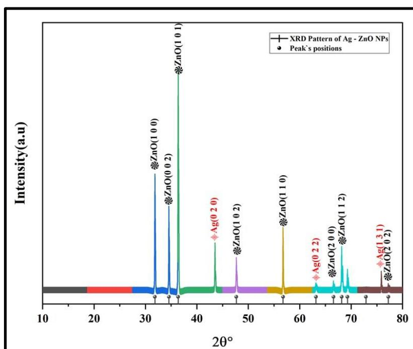
Fig. 3. X-ray diffraction patterns of silver and zinc nanocomposite prepared from *C. murale* extract after 24 h.
