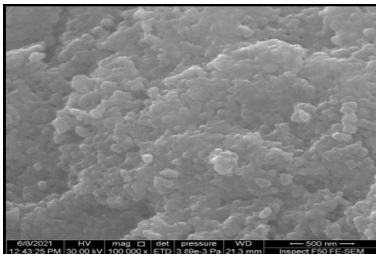
Fig. 4. The shape of the Ag: ZnO nanocomposite under a scanning electron microscope, the magnification power is 100,000X.
