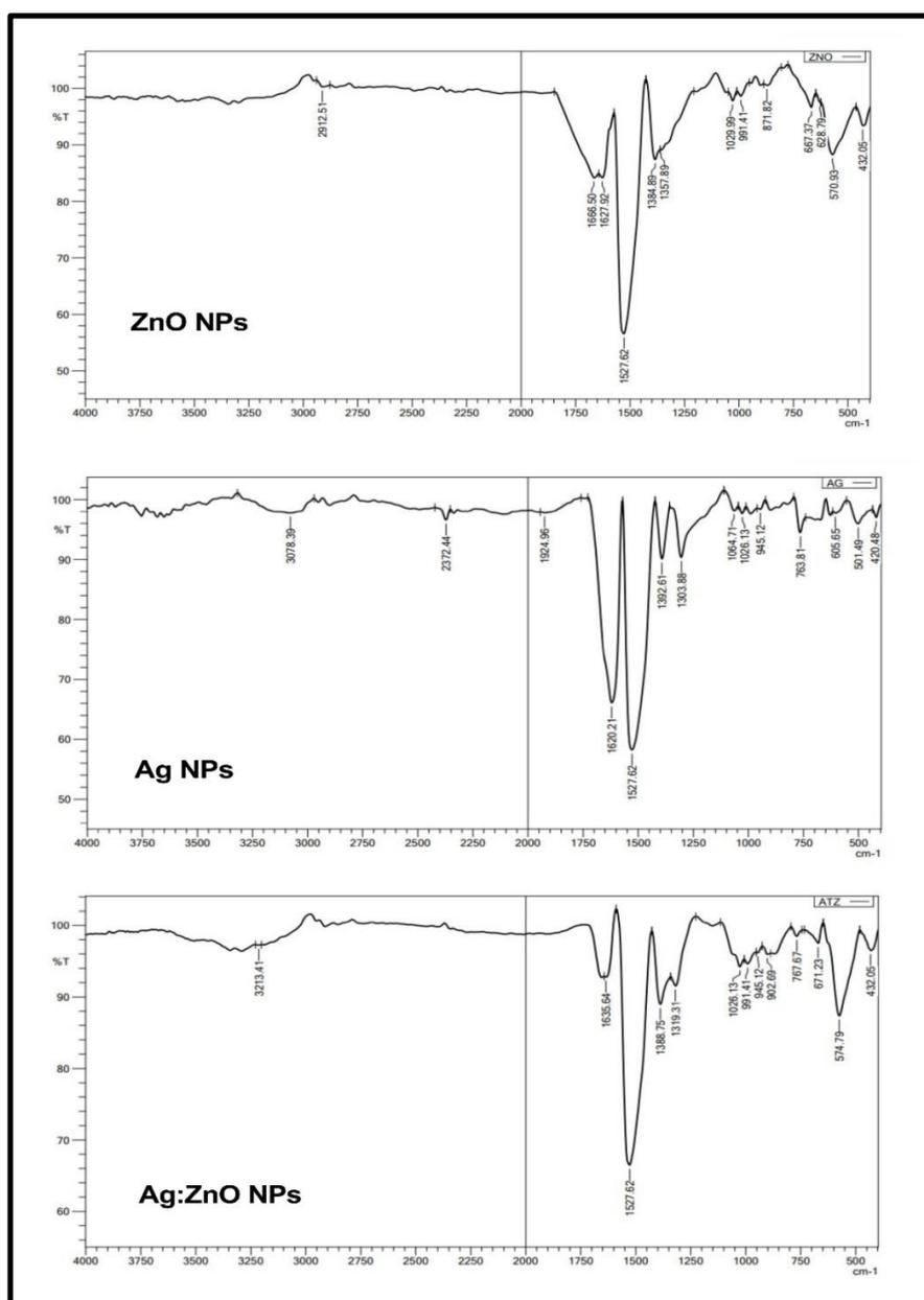
Fig. 2. FT-IR absorption spectrum of ZnO, Ag, and Ag: ZnO nanocomposite particles from 500 nm to 4000  $\text{cm}^{-1}$ .
