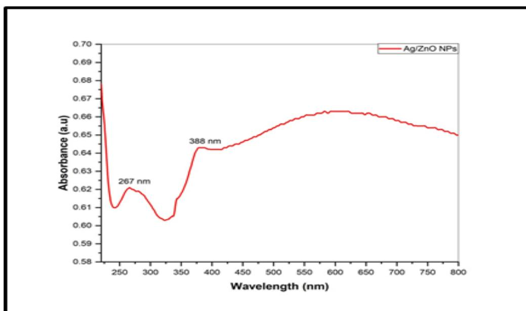
Fig. 1. UV absorption spectrum of Ag:ZnO nanoparticles from 200 nm to 1000 nm.
