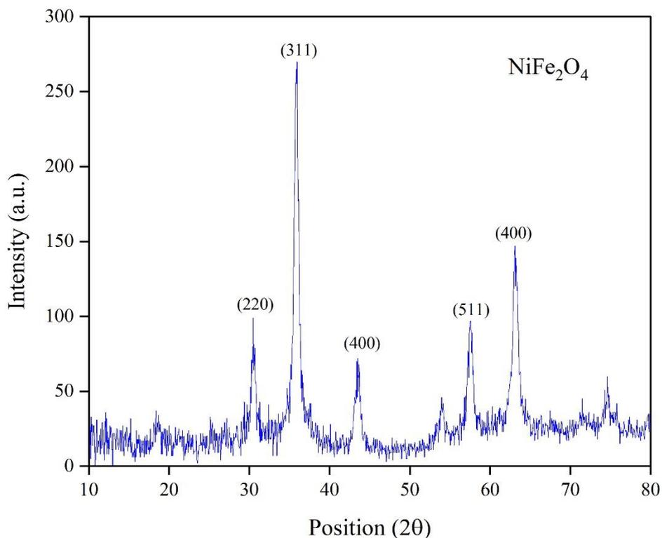
Fig. 1. XRD patterns of prepared NiFe<sub>2</sub>O<sub>4</sub> nanoparticles.
