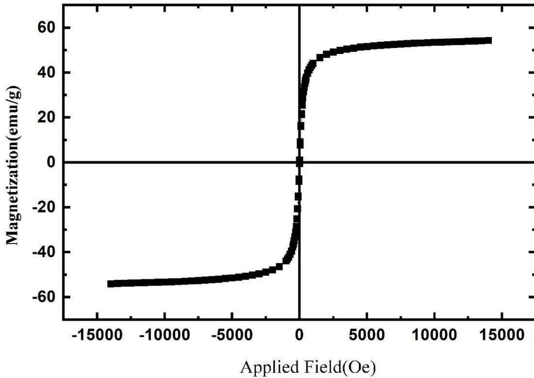
Fig. 5. VSM analysis of synthesized NiFe<sub>2</sub>O<sub>4</sub> nanoparticles
