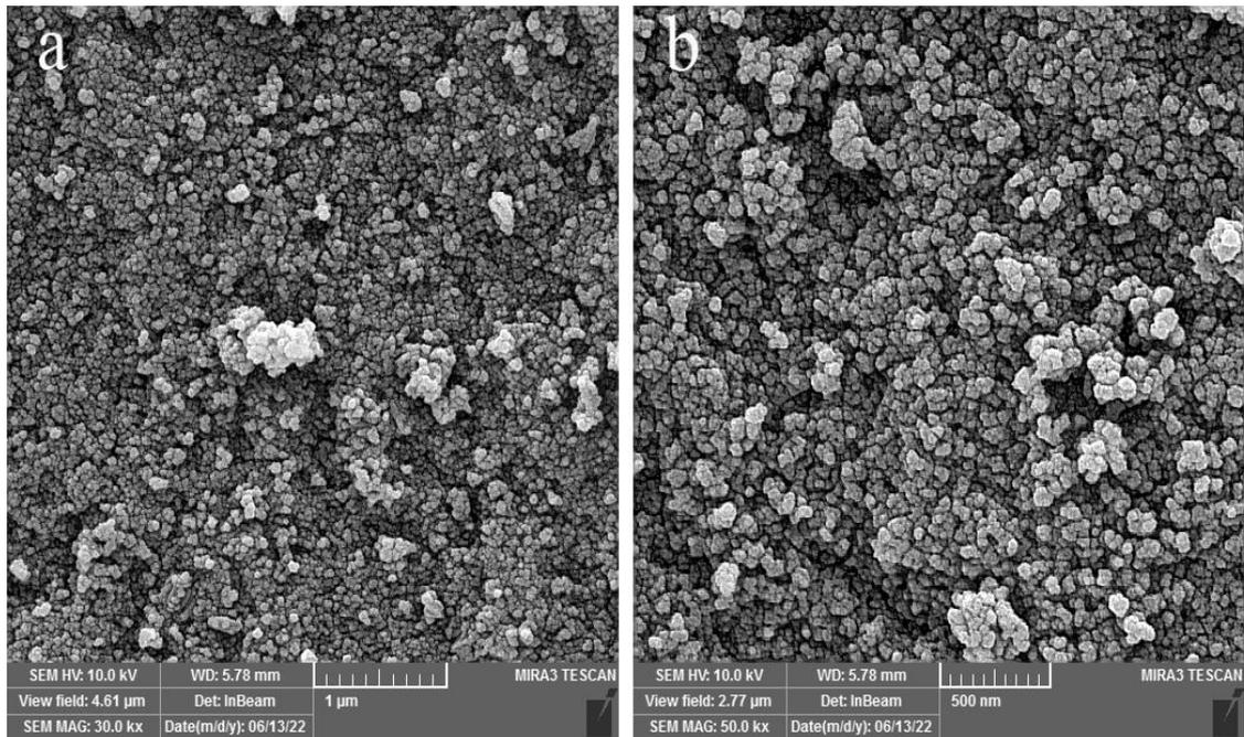
Fig. 3. SEM images of prepared NiFe<sub>2</sub>O<sub>4</sub> nanoparticles at different magnifications.
